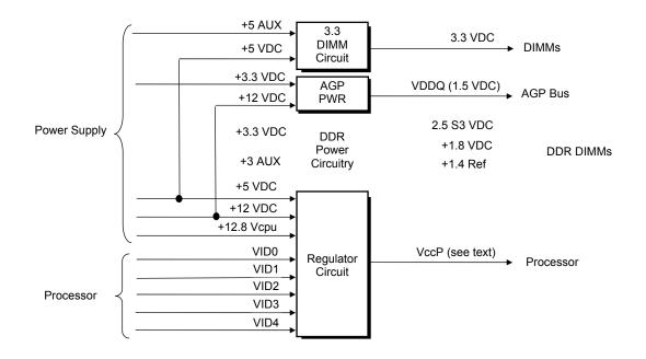
Figure 6–4. Low Voltage Supply and Distribution Diagram
